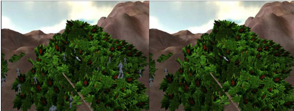
Figure 7. (left) all passes are rendered with CHC. Note that the soldiers are visible through the tree. (right) Only the solid passes are rendered using CHC, afterwards the transparent passes.
