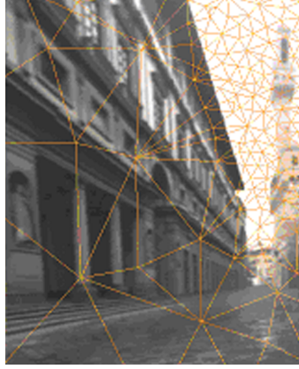
Figure 5.3: Final Delaunay grid on high dynamic range image. The centers of Voronoi cells are the sample points.
