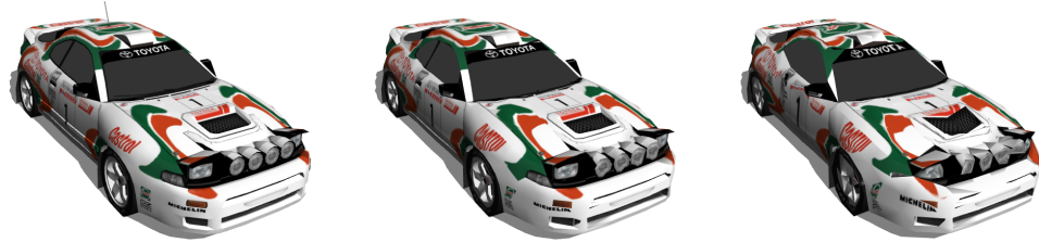
Figure 9.2: Example of geometry simplification. From left to right, the original object, the object simplified to 66% and the object simplified to 33%, respectively.
