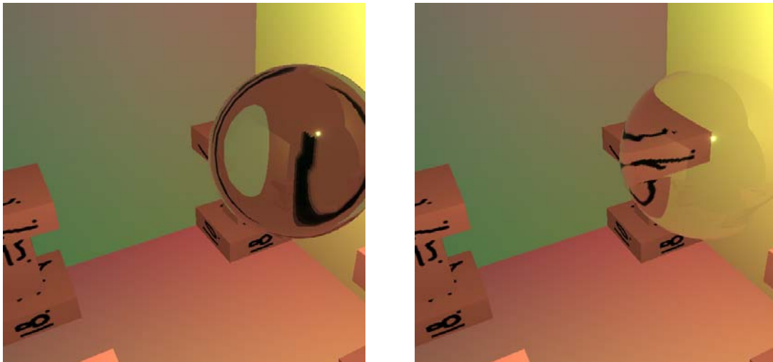
Figure 17. Refraction with classical environment mapping is highly inaccurate (left), our method works fine for this purpose, too.
