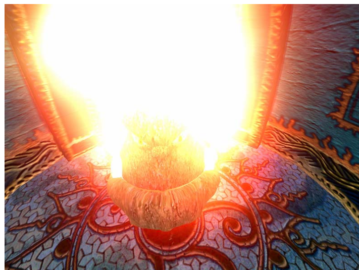
Figure 23. Spherical billboards implemented in Ogre. The demo shows an ogre head inside a particle system. Clipping and popping artifacts were removed by the spherical billboards method described in details in the GameTools technical documentation deliverable. Also a glow effect was added to the scene (see 2.6.1).
