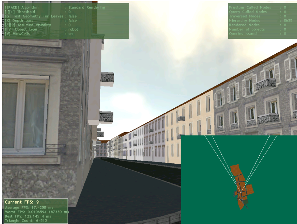
Figure 1, The PVS Computation Module integrated in the Ogre3d engine. A snapshot of Vienna is shown, with the rendered PVS shown in the lower right corner. Note how the PVS closely fits to the geometry actually seen.
