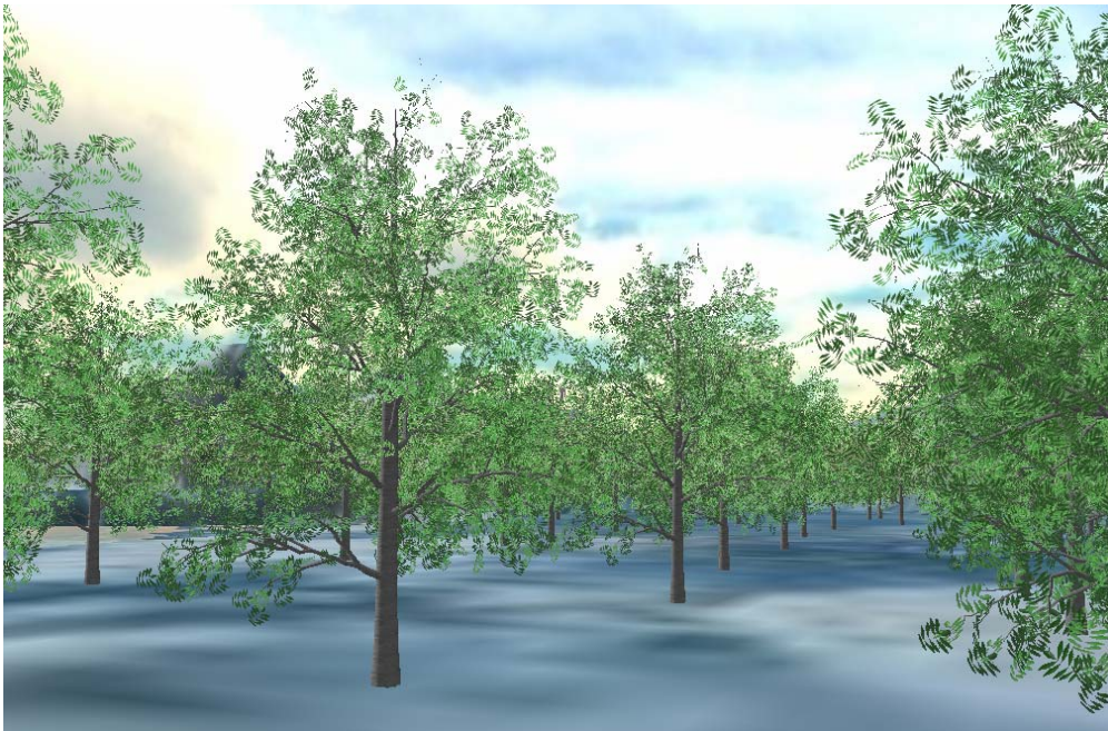
Figure 14: An LOD forest. The further is the tree, the lower the level of detail
