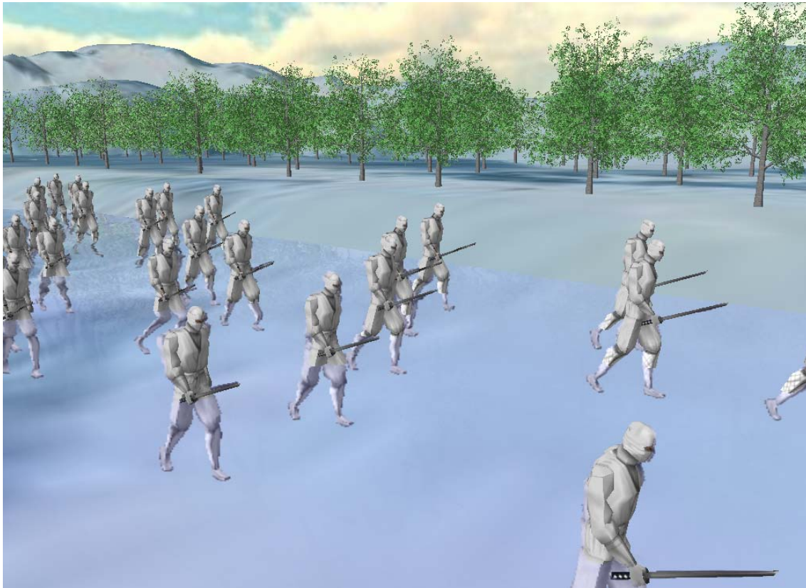
Figure 17: A complete LOD scene: LODStrips models (ninjas) in front of a LODTree-based forest
