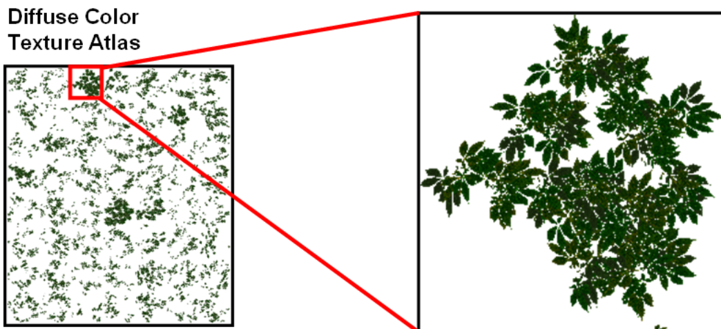
Figure 1.7: Diffuse color texture atlas that contains all the billboard textures. This texture atlas is used in the Standard texturing technique .
