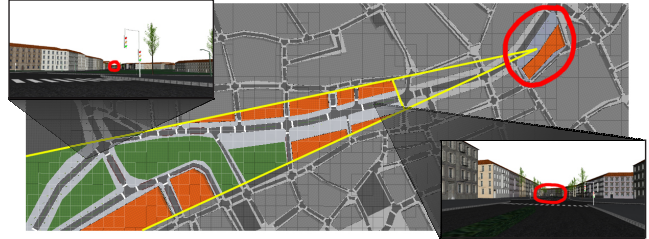
Figure 1: Example of automatic impostor placement (with the impostor in the circle, shown together with its shaft of validity).
