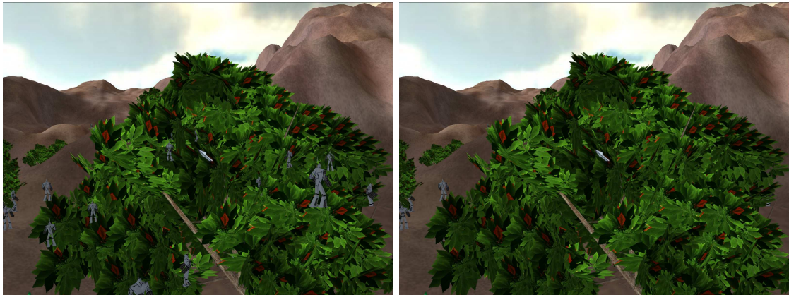
Figure 3.6: (left) all passes are rendered with CHC. Note that the soldiers are visible through the tree. (right) Only the solid passes are rendered using CHC, afterwards the transparent passes.
