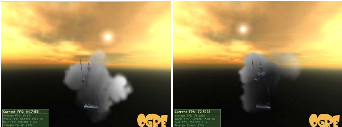
Figure 11. Hierarchical particle system with self-shadowing.
