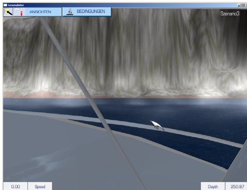
Spherical Billboards using depth information of the depth buffer
